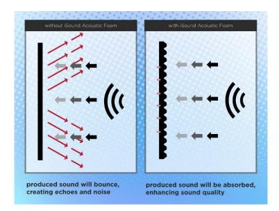
Figure 2.1 How acoustic foam works
