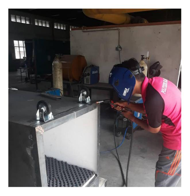
Figure 3.3.3 Welding the wheels behind the Sieve O' Sound
