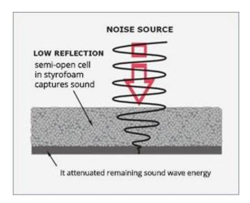
Figure 2.2 How Styrofoam respond to soundwaves
