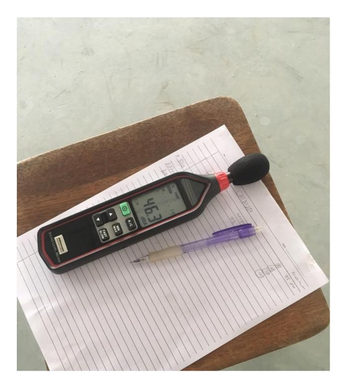
Figure 4.2.3 One of room reading taken by using Sound Level Meter.
