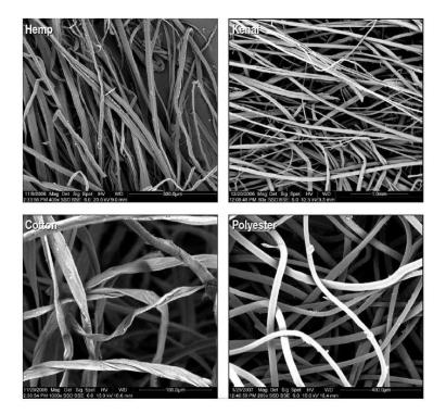
*Figure 2.4* Scanning electron microscope images on hemp samples, kenaf, cotton and polyester fibres. (Muller-BBN, Thermal Hemp 045, Measurement of Sound Absorption in the Reverberation Room According to DIN EN ISO 354, Test Report M52 297/1, Marc 2006)
