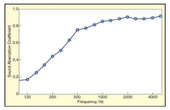
Graph 2.4 Graph showing the value of sound absorption coefficient that is carried out on cotton fibres. (Jorge P. Arenas & Malcolm J. Crocker "Recent Trends in Porous Sound-Absorbing Materials" Sound and Vibration, July 2010, Pages 12-16)
