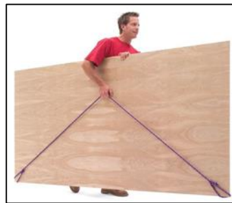
Figure 2.10: How to carry plywood with loop of rope.
