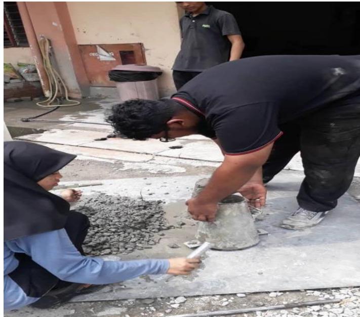
Figure 3.6 slump test of concrete
