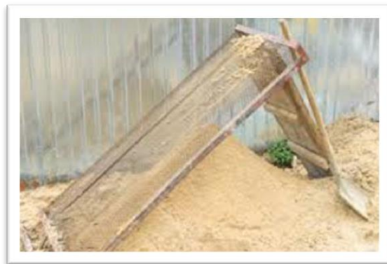
Figure 2.1 Traditional sand filter
