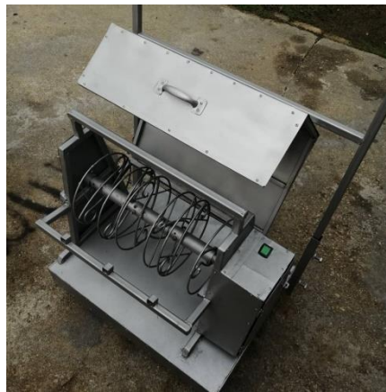
Figure 3.4.1 vi: Install switch and motor to function the roller and finishing the product with painting spray.
