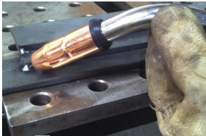
Figure 3.4: MIG welding on mild steel
