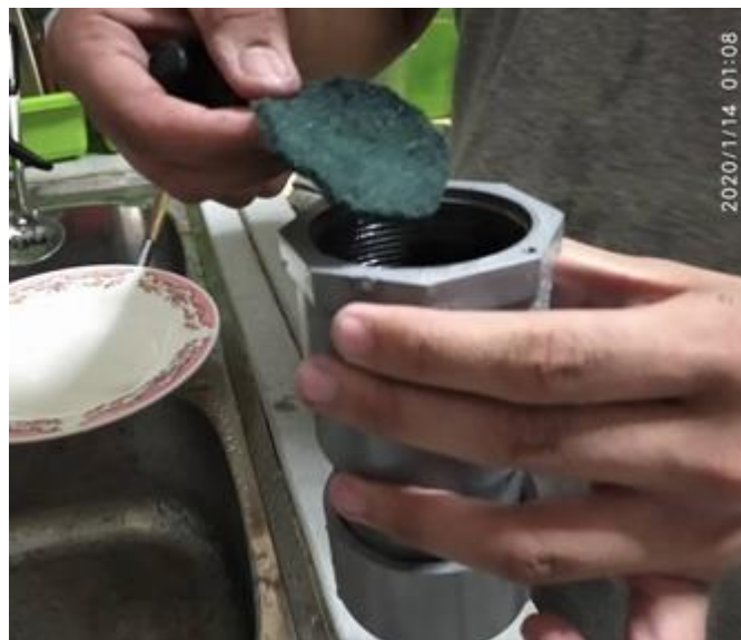
Figure 3.5 Nylon Pad on Filter Cylinder
