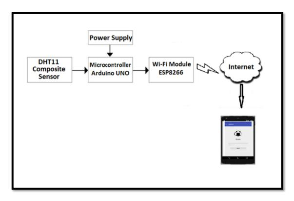
Figure 3. 2: Block diagram of the Project
