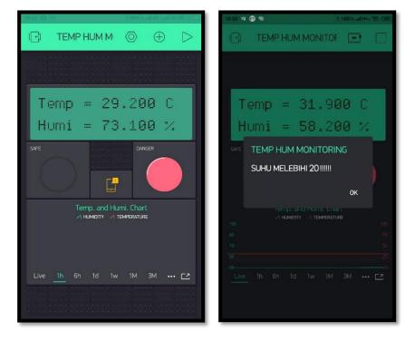
Figure 4. 4: Blynk with the Alert Notification
