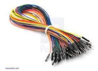
A jump wire is an electrical wire, or group of them in a cable, with a connector or pin at each end, which is normally used to interconnect the components of a breadboard or other prototype or test circuit, internally or with other equipment or components, without soldering.
