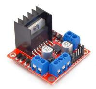
The L298N is an integrated monolithic circuit in a 15- lead Multiwatt and PowerSO20 packages. It is a high voltage , high current dual full-bridge driver designed to accept standard TTL logic level sand drive inductive loads such as relays, solenoids, DC and stepping motors
