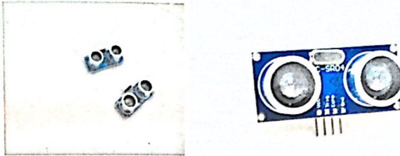
3.3.2 HC-SR 04 Ultrasonic sensor
