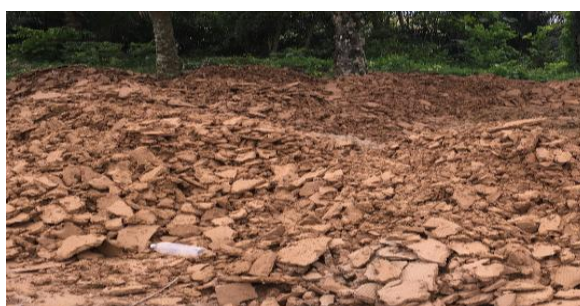
Figure 1 <Sludge Resulting from Water (River) Treatment Process>
