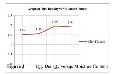
Figure 3 shows the maximum dry density and optimum moisture content for the clay soil mixed with fly ash are  $1.95g/m^{3}$  and 22%.
