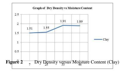
Figure 2 shows the maximum dry density and optimum moisture content for the native clay soil are  $1.91g/m^2$  and 33%.
