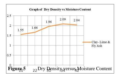
Figure 5 shows the maximum dry density and optimum moisture content for the clay mixed with lime and fly ash are  $2.09g/m^3$  and 34%.
