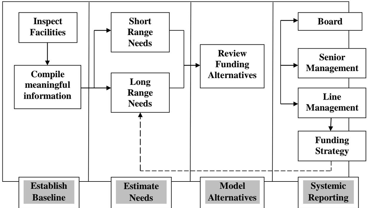
Figure 2.1: Facility Condition Assessment Process
