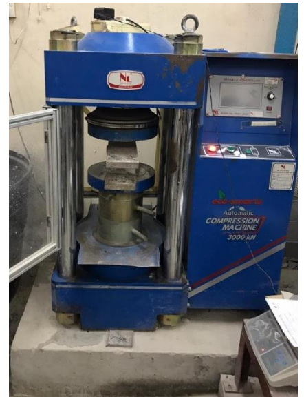
COMPRESSIVE STRENGTH TEST
