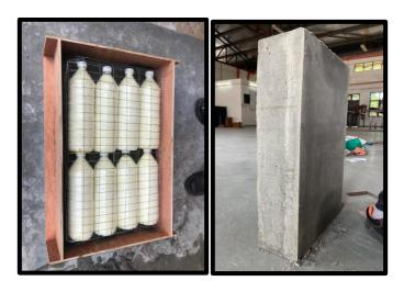
Figure: lightweight wall panel prototype has been replaced with bottle plastic filled with foam (pu200) as a brick
