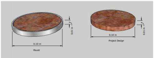
The research design of our project is we using a circle mould with diameter of 10 cm to put the crushed banana stems. The measurement of the design is 10 cm of the diameter with 1 cm of the mould thickness. On the right diagram is the product. The product is put into a glass that fill with 300 ml of water that mix with the oil.
