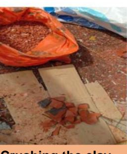
Crushing the clay rooftiles into grain size particles.
