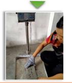
The bricks weight was recorded to obtain water absorption
