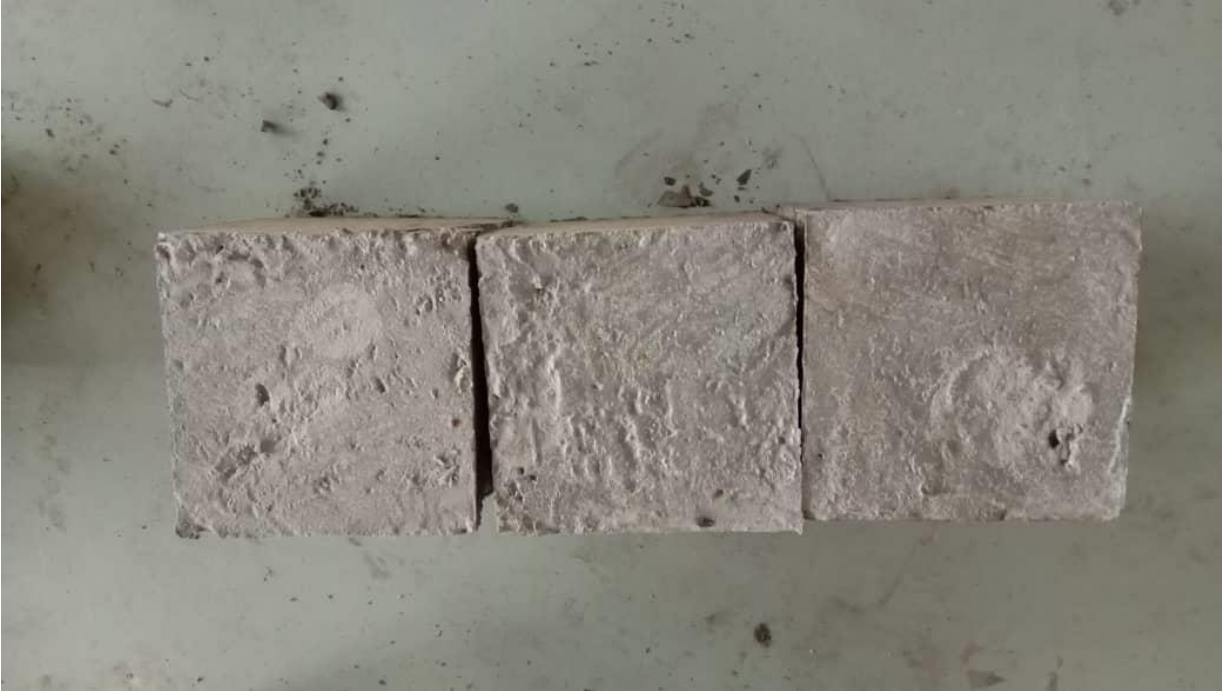
Figure 1: Concrete samples that has been replaced by recycle ceramic tiles with 5% replacement.
