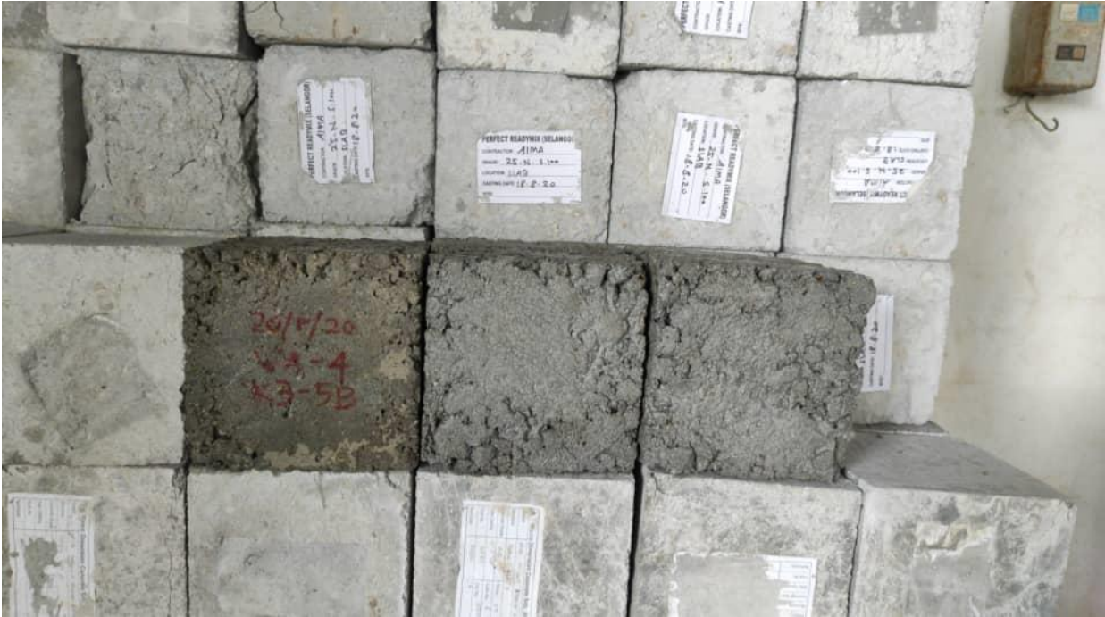
Figure 2: Condition of concrete samples after Compressive Strength test.
