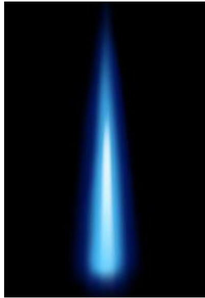
Figure 2.4.4: Complete combustion of LPG
