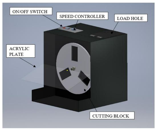
Figure 3.13: Machine Detail
