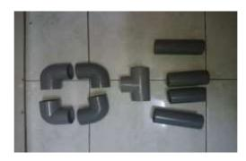
Figure 3.3.2 – PVC PIPE CONNECTOR AND COUPLING SET
