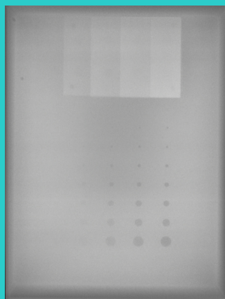
Common x-ray Test Object, Lucite Plastic Board
