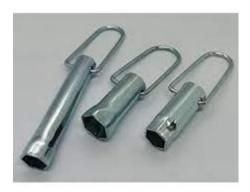
The most important tool is a spark plug socket. Spark plug sockets come in two sizes which is 5/8 and 13/16 inches. Most afternarket spark plug sockets have a rubber insert that holds the plug in place.
