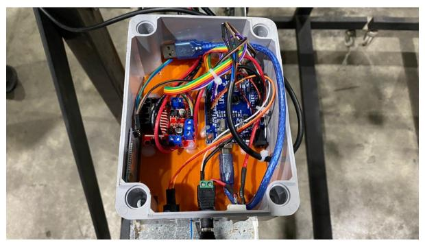
As we can see the above, it was the casing for the product that made of using 3D printing method. With all the measurement of the casing, we had put and arrange the Arduino board and the sensors.
