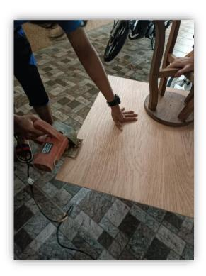
The process of cutting plan wood after being measured is set
