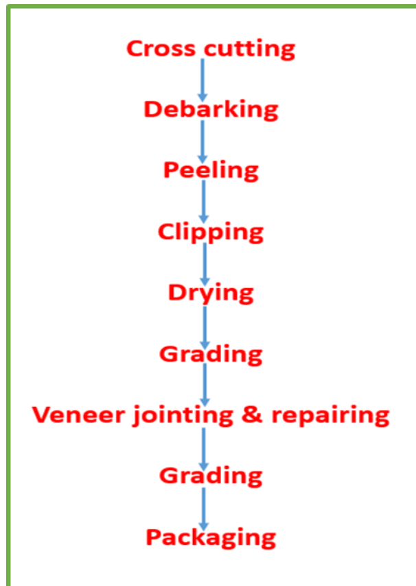
Diagram A1(c): Veneer Production Flow chart Gambar rajah A1(c): Carta alir pengeluaran venir
