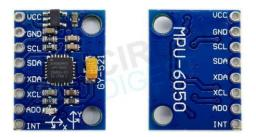
MPU6050 is a Micro Electro-mechanical system (MEMS), it consists of three-axis accelerometer and three-axis gyroscope. It helps us to measure velocity, orientation, acceleration, displacement and other motion like features. MPU6050 consists of Digital Motion Processor (DMP), which has property to solve complex calculations.
