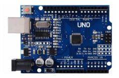
Arduino/Genuino UNO is a microcontroller board based on the ATmega328P. It has 14 digital input/output pins (of which 6 can be used as PWM outputs), 6 analog inputs, a 16 MHz quartz crystal, a USB connection, a power jack, an ICSP header and a reset button. It contains everything needed to support the microcontroller.
