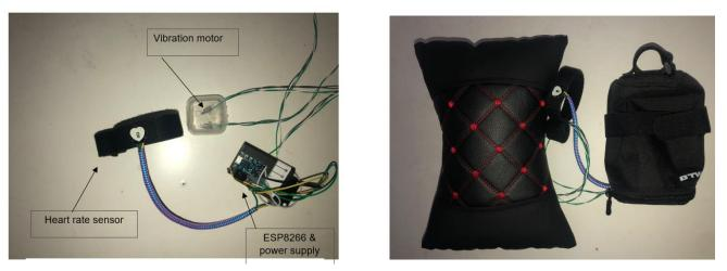
FIGURE 15: The result of microsleep detect and alert system for driver project prototype
