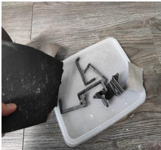
Figure 3.2.3: shows the progress of rough sanding process
