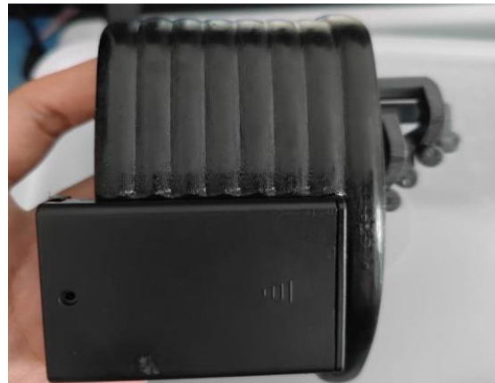
Figure 3.4.7 shows the protective cover after sprayed 3 layers of clear coat.
