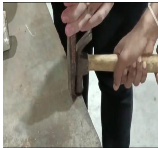
Figure 3.2.4: shows the progress of metal pin cutting process
