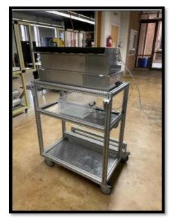
Cart Assembly with Humidifier Facing Out
