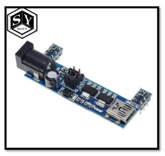
FIGURE 3.5 : Power Module MB-102
