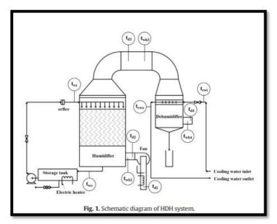
Schematic diagram of HDH system.
