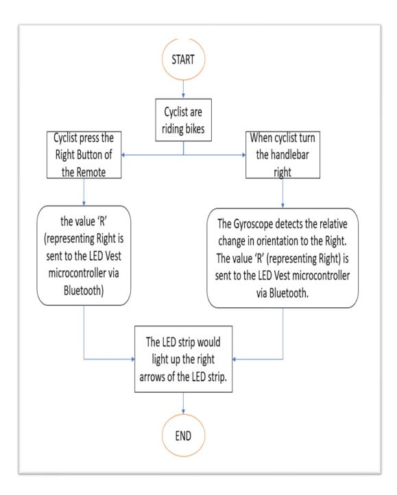
Figure 3.1: Flow chart of operation of the system
