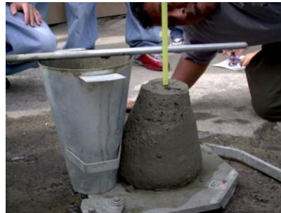
Diagram 3.14 Slump test concrete (pinterest.com).
