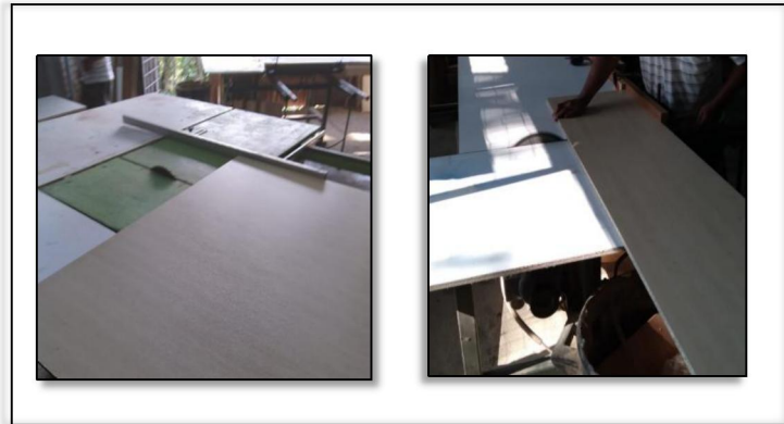
Figure 3.7 Cut the Chipboard by using Table Saw
