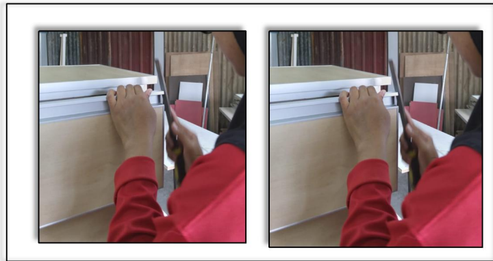
Figure 3.10 A chisel is used to flatten the surface of the aluminum edge tape
