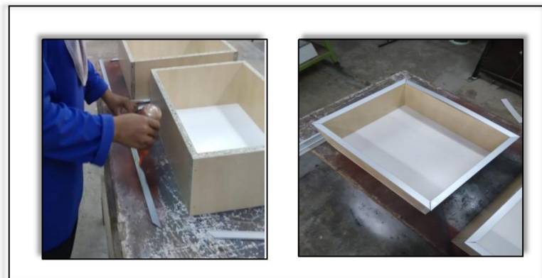
Figure 3.8 Applied wood glue and aluminium edge tape
