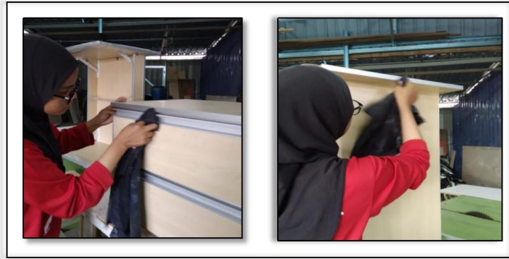
Figure 3.9 Applied mineral turpentine to to remove any residue left behind
