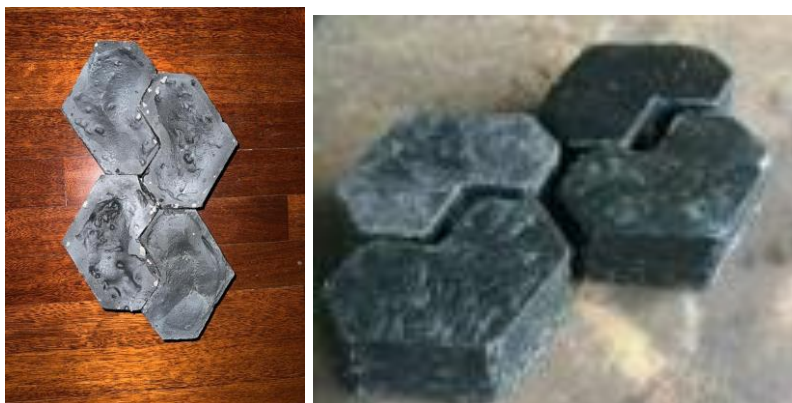
Figure 3.12: Final product of recycle interlocking brick
