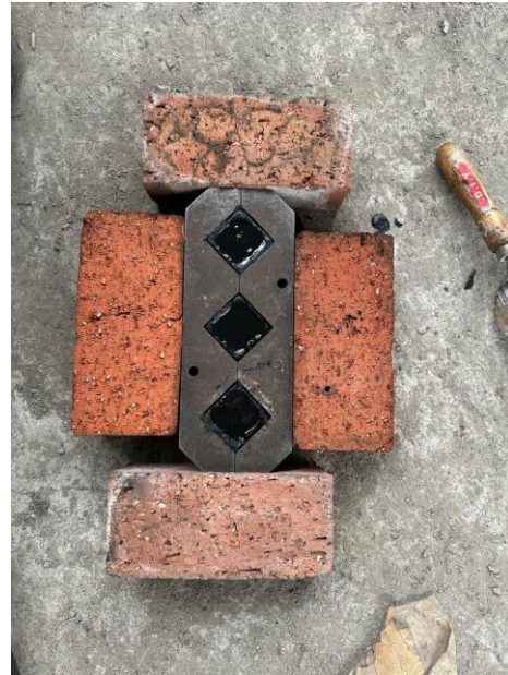
Figure 3.8: Transfer the mixed into cube test (50mmx50mmx50mm)
