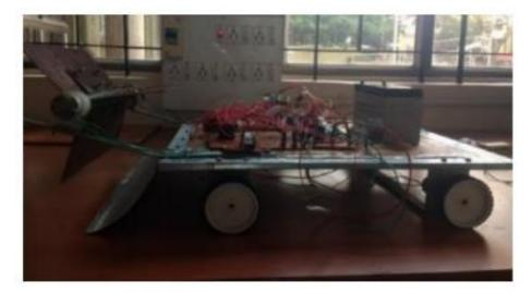
The blades of this trash collection system revolve around a shaft that is attached to the motors. The mechanism will only activate when necessary and not for the whole of the vehicle's operation. With some consideration for ground clearance, this collection device is installed on the front side. To perform the rotating mechanism, two motors are installed on the two sides of the shaft and connected to Arduino.
