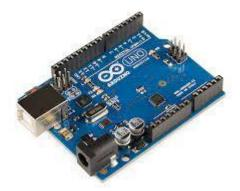
Arduino UNO is a microcontroller board based on the ATmega328P. It has 14 digital input/output pins (of which 6 can be used as PWM outputs), 6 analog inputs, a 16 MHz ceramic resonator, a USB connection, a power jack, an ICSP header and a reset button.
