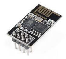
The ESP8266 WiFi Module is a self contained SOC with integrated TCP/IP protocol stack that can give any microcontroller access to your WiFi network. The ESP8266 is capable of either hosting an application or offloading all Wi-Fi networking functions from another application processor.
