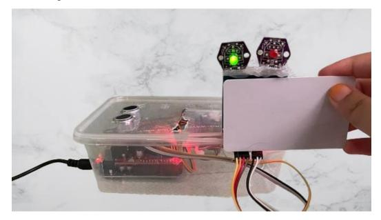
when the user has finished scanning and the green light has gone out, the user can use the parking lot
