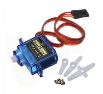
A **servo motor** is a type of motor that can rotate with great precision. Normally this type of motor consists of a control circuit that provides feedback on the current position of the motor shaft, this feedback allows the servo motors to rotate with great precision. If motor is powered by a DC power supply then it is called DC servo motor, and if it is AC-powered motor then it is called AC servo motor.
