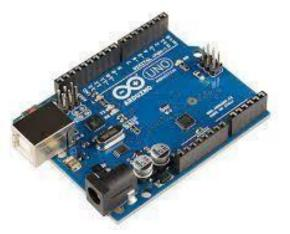
Arduino Uno R3 board, Arduino is an open-source physical computing application based on a basic I / O board and a programming framework that incorporates the Processing / Wiring language .The Arduino will be a
