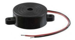
An audio signaling device like a beeper or buzzer may be electromechanical or piezoelectric or mechanical type. The main function of this is to convert the signal from audio to sound. Generally, it is powered through DC voltage and used in timers, alarm devices, printers, alarms, computers, etc. Based on the various designs, it can generate different sounds like alarm, music, bell & siren.
