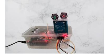
The below diagram shows the status of the parking zone when the auditor scan on the RFID reader using the correct card, the green LED will light up and the barrier will go down
