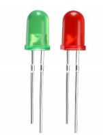
The Bi-color LED is a handy little component that allows two colors (red and green) in a single LED while only having two pins (cathode and anode). The
