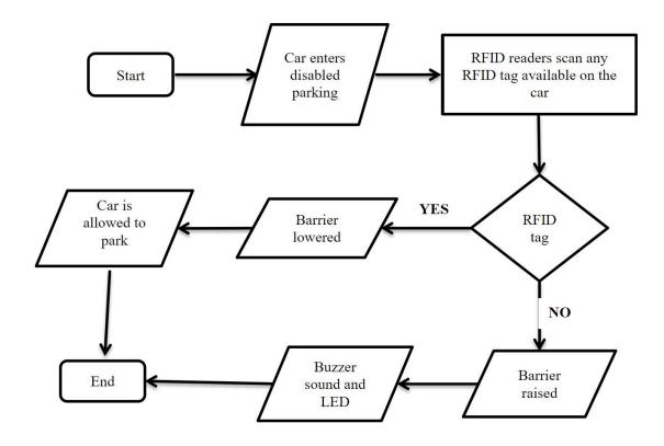
Figure 3:2 Flowchart of operation of the system
