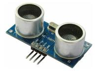
An ultrasonic sensor is an instrument that measures the distance to an object using ultrasonic sound waves.
