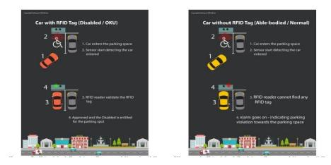
Figure 2:1 image of different between use RFID tag and no RFID tag
