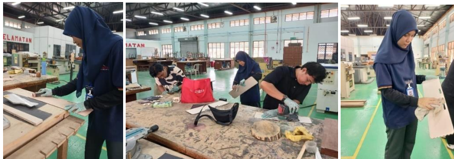
Figure 3.16 Manual sanding and using a palm sander, followed by wiping off dust with a cloth. The sanding and wood filler application steps were repeated twice on each side
