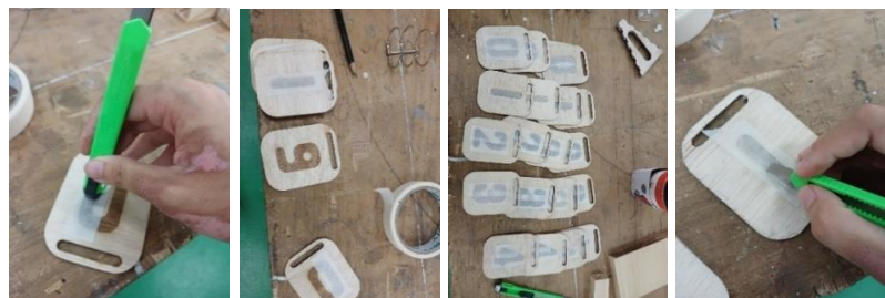
Figure 3.14 Initial stages of covering the parts where wood filler isn't needed
