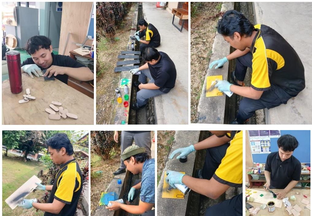
Figure 3.19 Repeat sanding before applying spray paint. Each part is then spray painted according to the predetermined colours. Once dried, veneer is applied.
