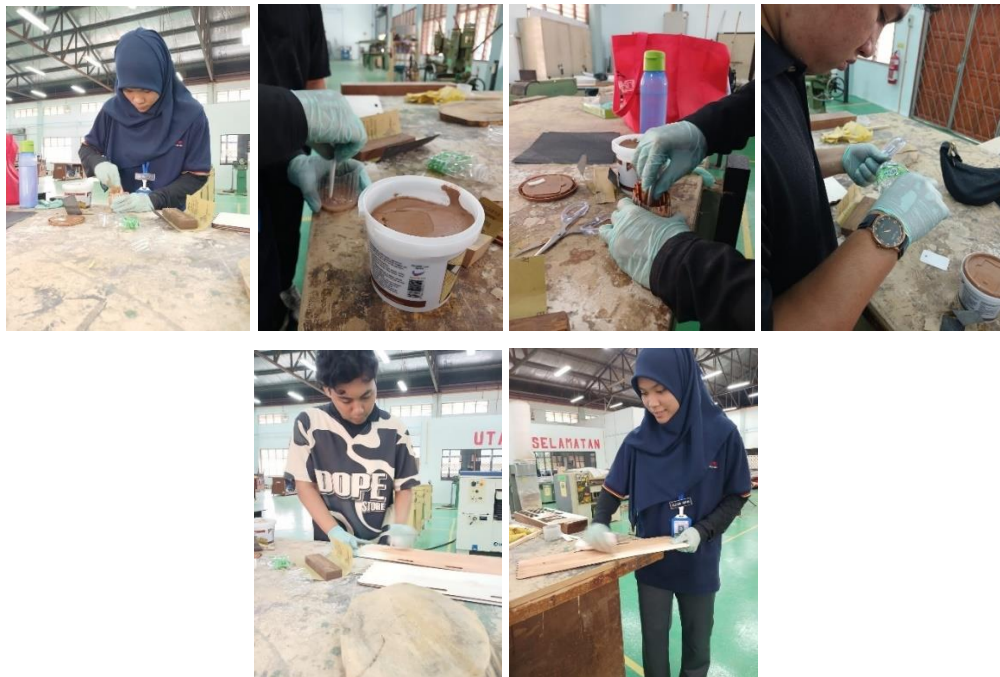
Figure 3.15 Mixing wood fillers with water, then applying it to the surface of plywood
