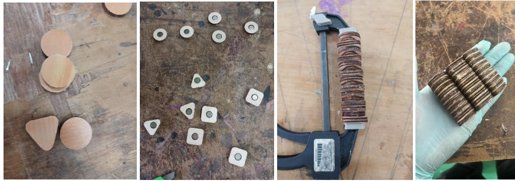
Figure 3.18 Apply glue to the veneer and put magnets in each part. Trim the remaining veneer and clamp it all together using quick-release clamps
