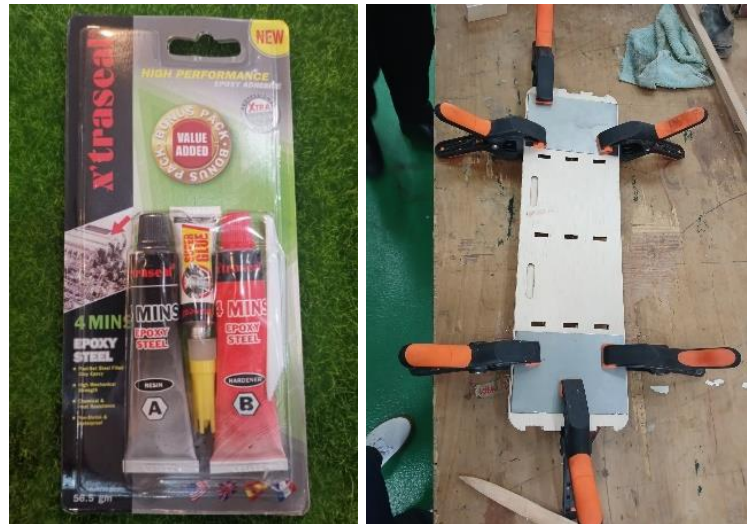
Figure 3.27 Epoxy and hardener were used to glued steel plates onto the back of the base
