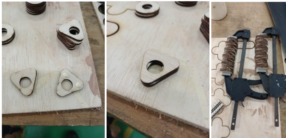
Figure 3.17 Gluing parts with wood glue, then clamp them using quick-release clamps
