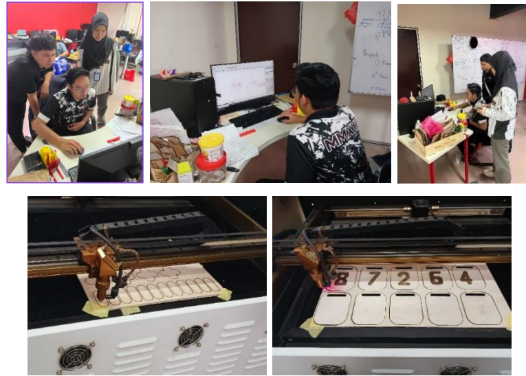
Figure 3.13 Cuts and engravings performed using the laser cutting and engraving machine under Alif's guidance
