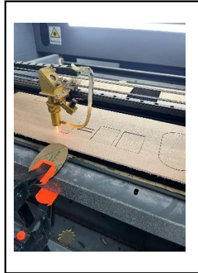
Rajah 96: Proses Laser Cutting
