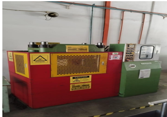
Mesin penekan panas 100 Tonne Hydraulic Laboratory Hot Press
