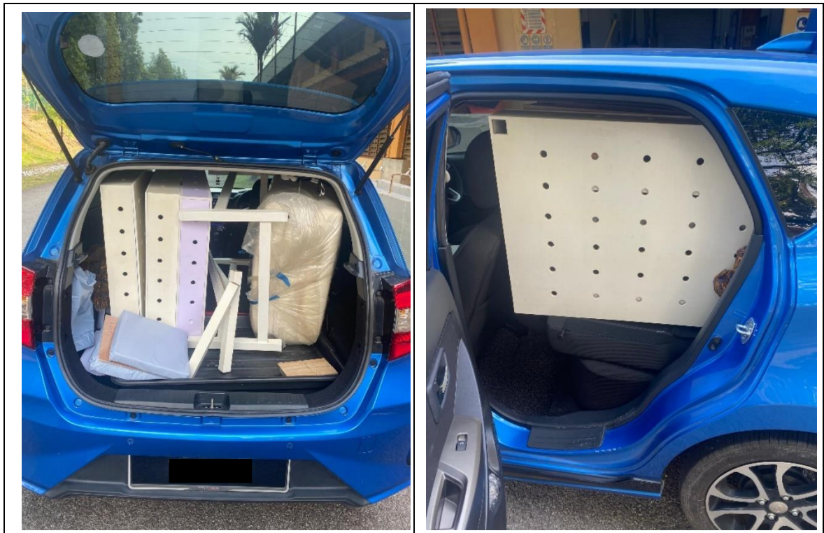
Figure 3. 14: Disassembled SANiBED form in a hatchback car
