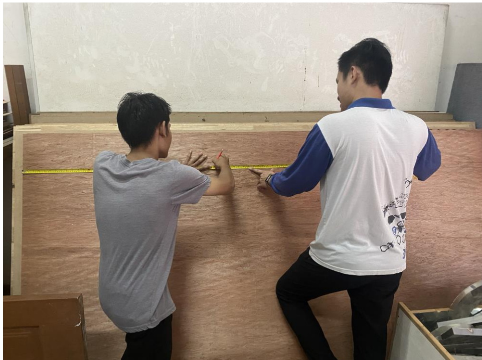
Figure 3. 6: Marking process on a plywood
