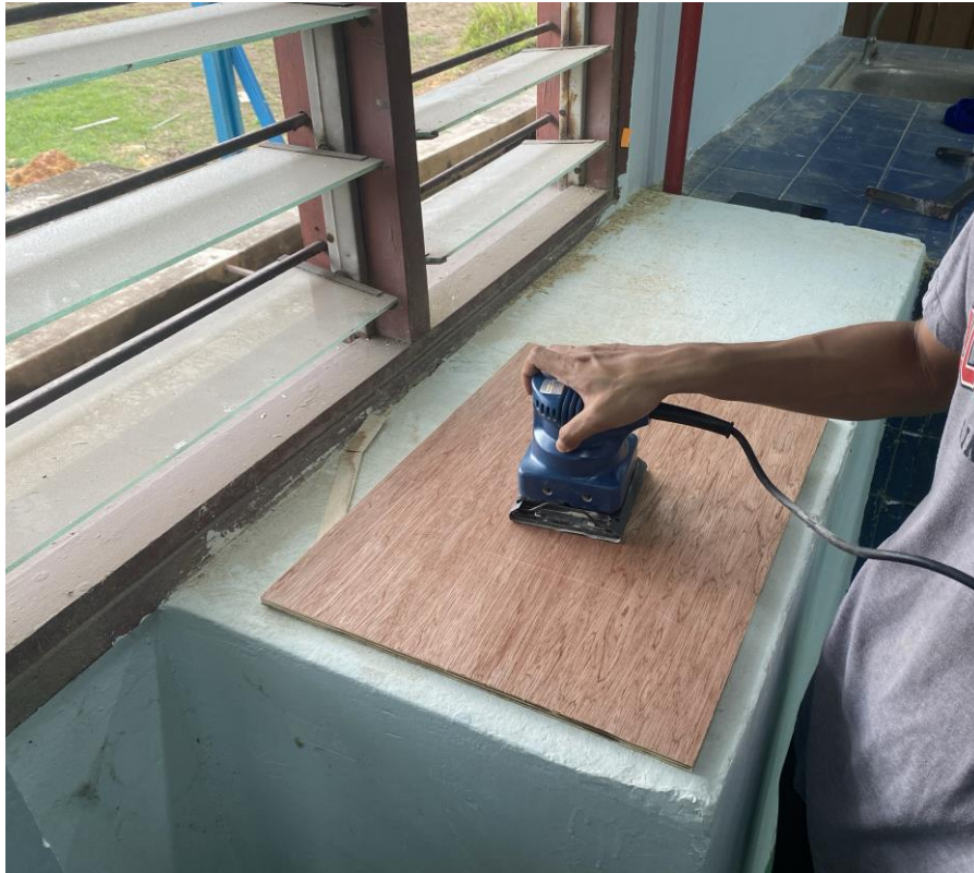
Figure 3. 9: Sanding process on the edge and surface of materials
