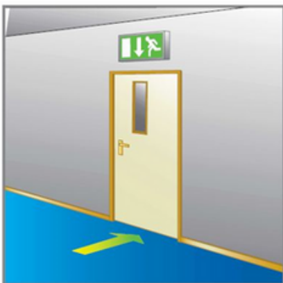
At each exit door
