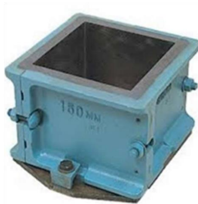
Figure 2.4.1: The Example Of Cube Mould With Length X Width X Height(150mm X 150mm X 150mm)
