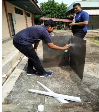
FIGURE 5: The product was colored with white spray as basement before colored with yellow.
