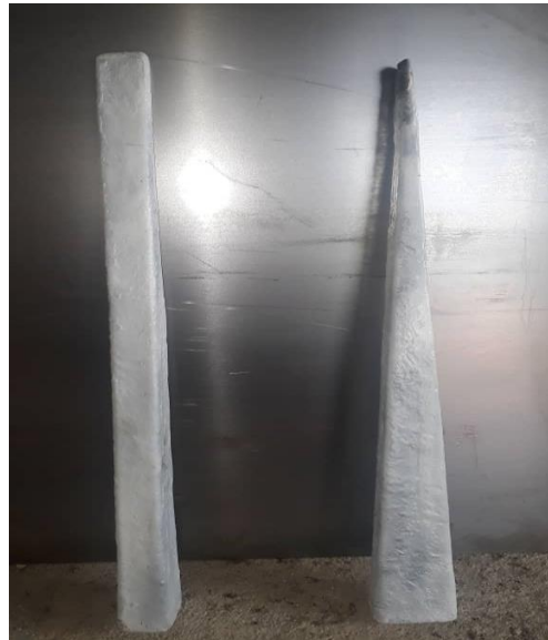
Figure 9: The wood that are coated with fiberglass
