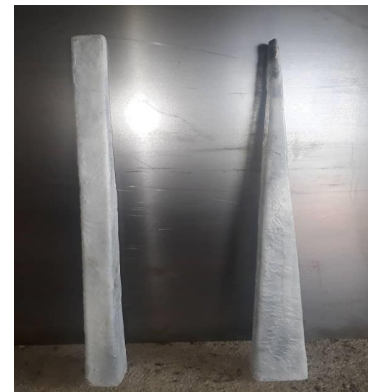
FIGURE 2: The balau wood coated with fiberglass.
