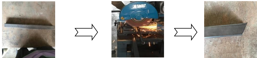
Figure 3.4.10 : cutting process to 45 degree
