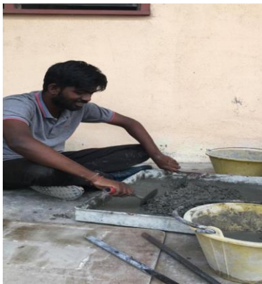
Materials are mixed according to the ratio and poured into the mould.
