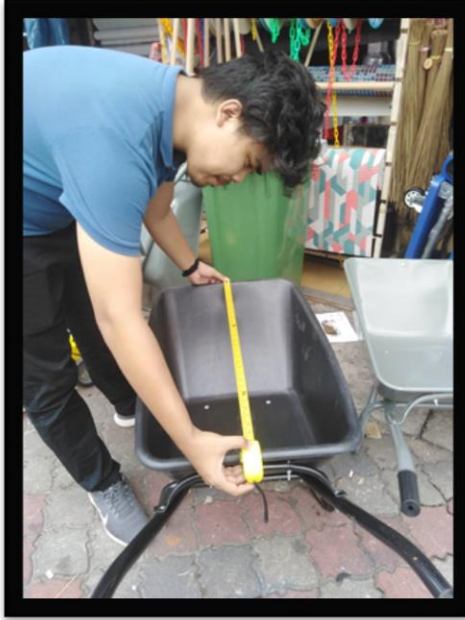
Figure 2.15 Length of the wheelbarrow's tray
