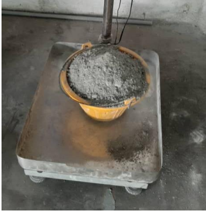
Figure 3.1: cement is being weight
