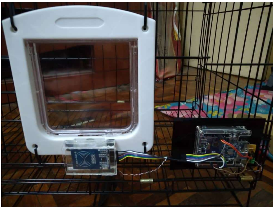
Figure 2.8 : New cat cage door with RFID
